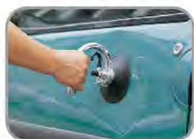
To pull up the plating notched part.
